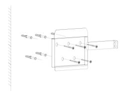
Figure 4-6 Fixing the wall bracket
