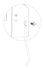
Figure 4-8 Grounding terminal connection
