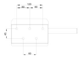
Figure 4-4 Dimensions of wall bracket
