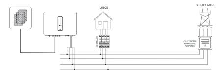
Figure 5-1 Electrical wiring diagram
