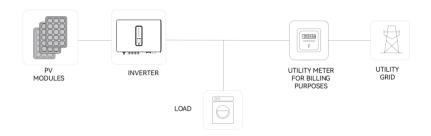
Figure 3-1 Schematic diagram of PV grid-connected system
