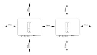
Figure 4-2 Recommended installation spacing
